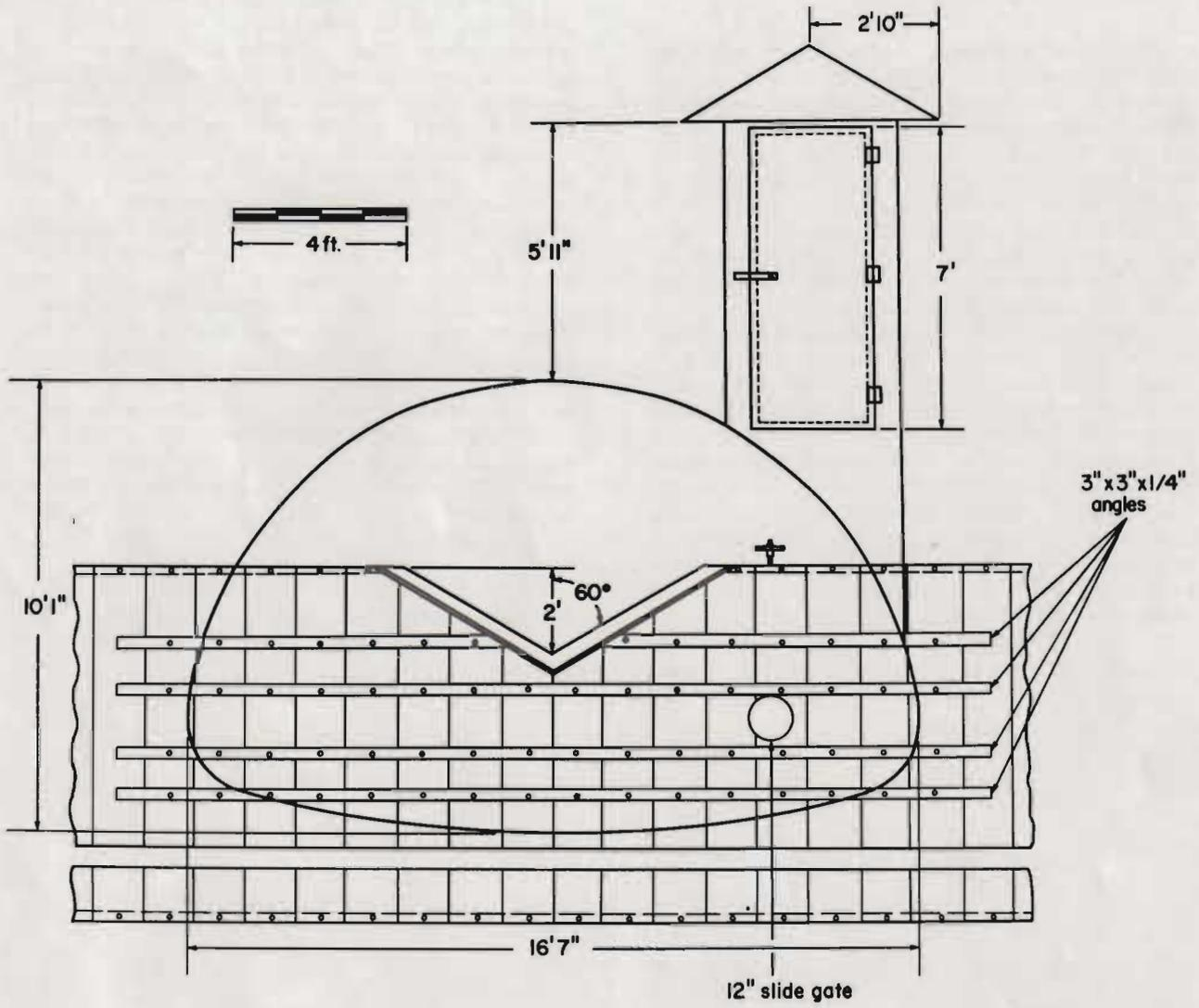
Figure 5.—Section B-B: view at cutoff wall of the enclosed weir.
