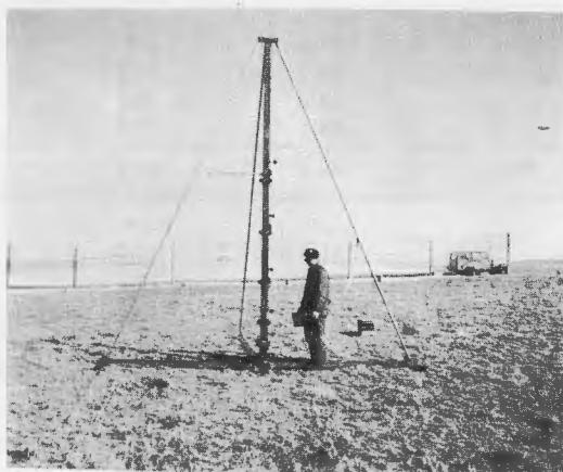
Figure 1. Portable mast 100 ft upwind of a 10 ft panel
