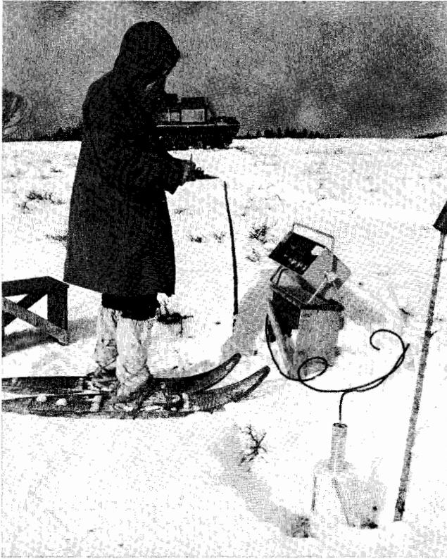
FIG. 1. Winter soil moisture measurements with neutron-probe equipment.
