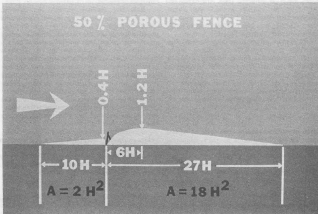
Figure 6. Ideally, a snow fence is 50-percent porous; a simple equation— $10 \times H^2$  (height of the fence)/lineal ft of fence—can be used to determine approximately the volume of water stored behind a snowfence.
